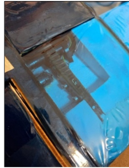
Figure 12, integrated angle sensor under skin
