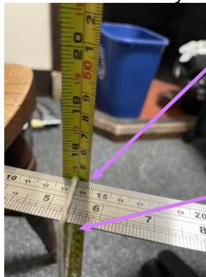
Figure 3 - Image showing how to position tape measure to measure distance to ground
