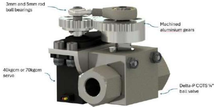
Figure 10 - 1/4" geared servo-valve
