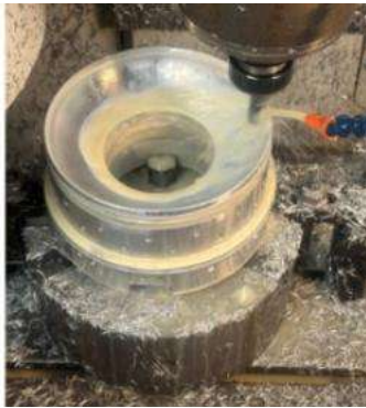
Figure 26: End cap machining
