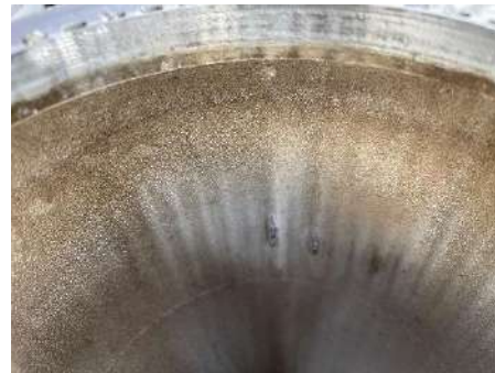
Figure 112 & 12, Swarf can be seen trying to escape through the burst channels
