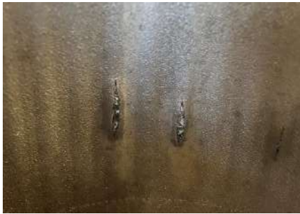
Figure 112 & 12, Swarf can be seen trying to escape through the burst channels
