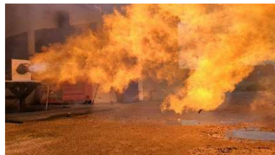
Figure 113 Hot fire data where the flame front was pushed out of the combustion chamber producing negligible chamber pressure.
