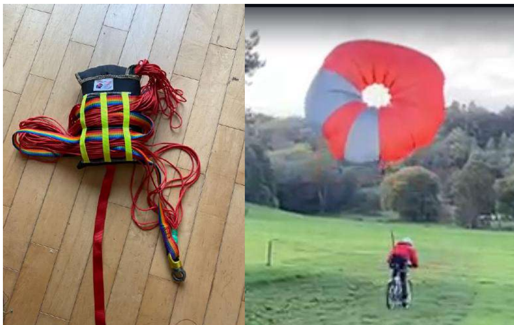
Figure 38 Left main chute packed into deployment bag, right demonstration of main parachute.
