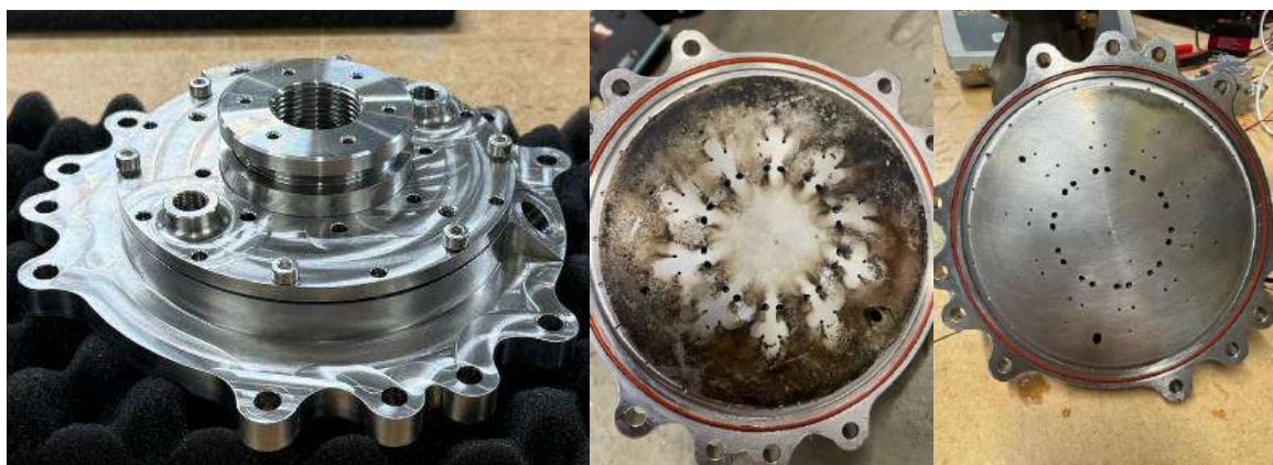
Figure 7 – (A) Assembled injector plate. (B) Deposits on injector plate following hotfire. (C) Cleaned injector plate following hotfire.
