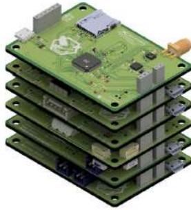
Figure 47: Avionics Stack Module Render
