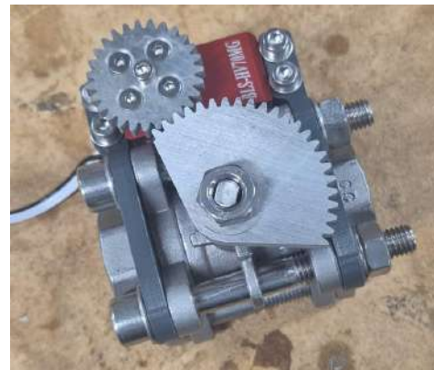
Figure 11 – Left: 3/4" geared servo-valve design in CAD Right: Assembled on the workbench.
