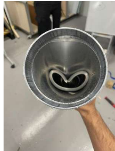
Axial view of tank buckling
