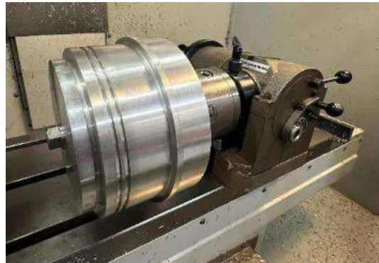
Figure 27: Dividing head for radial features
