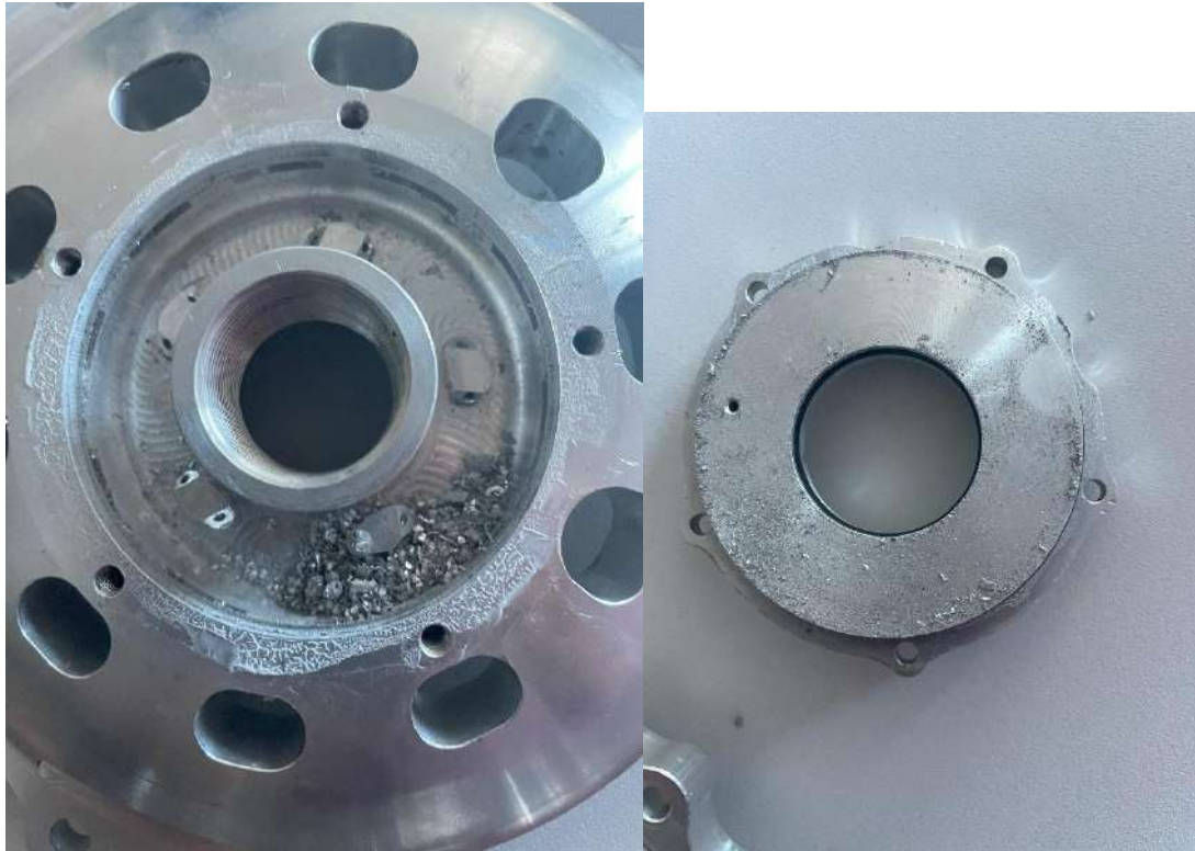
Figure 18 & 19, Injector fuel cap and fuel manifold after removal. Massive amounts of swarf deposited inside.
