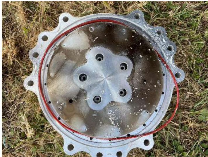
Figure 16, Injector plate immediately after it was taken off of the chamber. Swarf everywhere.
