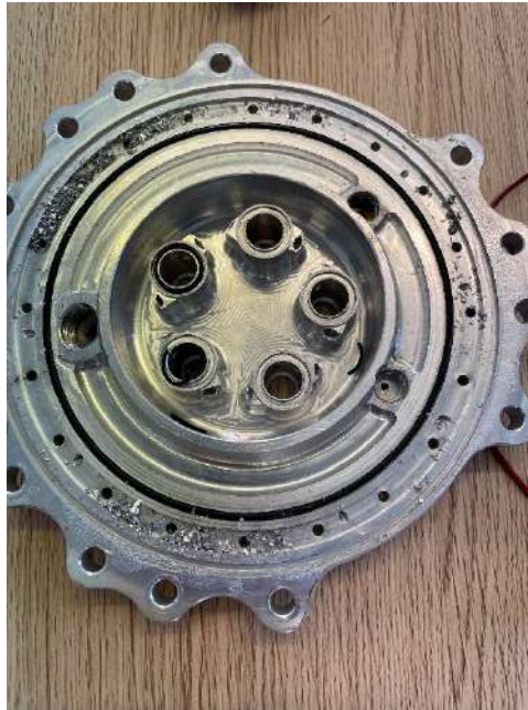
Figure 17, inside Injector. Swarf clearly visible in the fuel collection manifold. Swirl element O-rings broken and missing.
