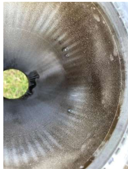
Figure 112 & 12, Swarf can be seen trying to escape through the burst channels
