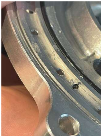
Figure 18, close-up of film cooling hole. Completely blocked by swarf.
