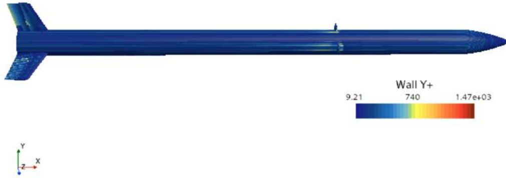
Figure: y^+ value along rocket length at 100% deployment at 80 m/s
