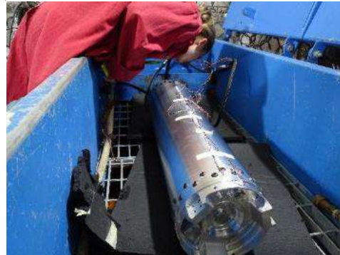
Figure 29: Post hydrostatic test inspection
