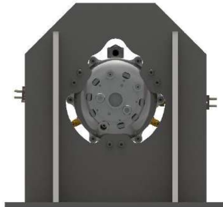
Figure 131: Bolthole locations within L-bracket
