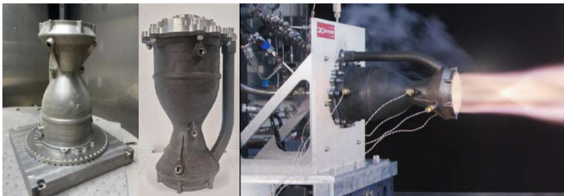
Figure 2 - ENGINE-1 Left: as printed on build plate Centre: as assembled with stainless steel injector; Right: photo from bench testing the engine producing 5kN thrust for a 3s burn, results detailed in Appendix B9.
