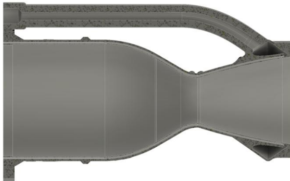
Figure 21: 1/2 section view of Engine-1 & regenerative cooling channel profile
