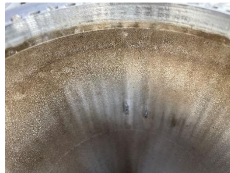
Figure 11 & 12, Swarf can be seen trying to escape through the burst channels
