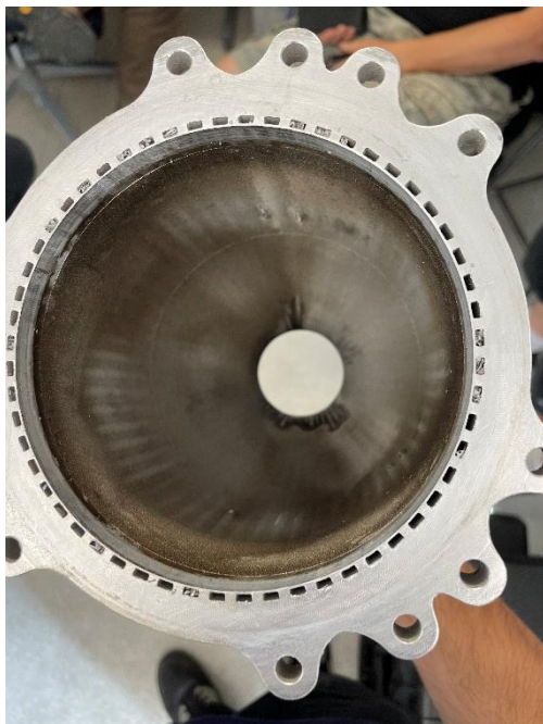
Figure 13 & 14, Channels are clearly filled with swarf. Popping and bursts clearly visible as well as throat melt streaks.
