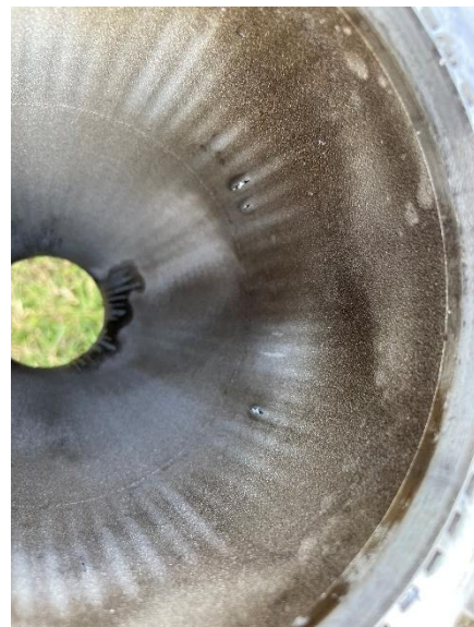
Figure 13 & 14, Channels are clearly filled with swarf. Popping and bursts clearly visible as well as throat melt streaks.
