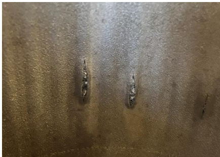
Figure 11 & 12, Swarf can be seen trying to escape through the burst channels
